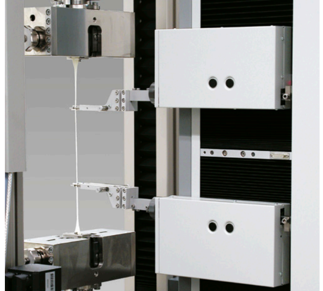
Fig. 2: The easy-change sensor arms are attached to the carriage-mounted measuring heads
