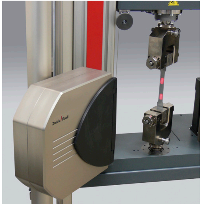
Fig. 2: LaserXtens with typical speckle pattern
