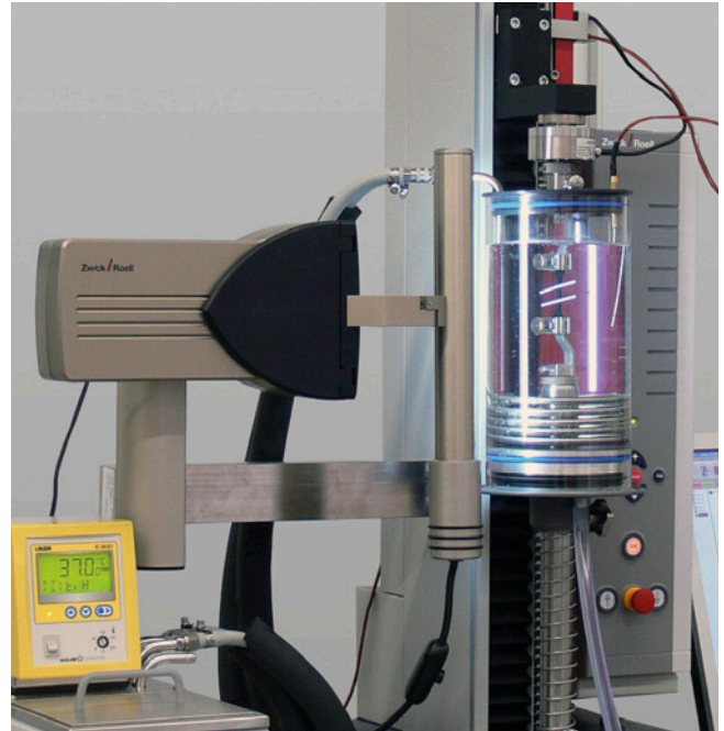
videoXtens - Non-contact measurement in a temperature-controlled fluid bath
