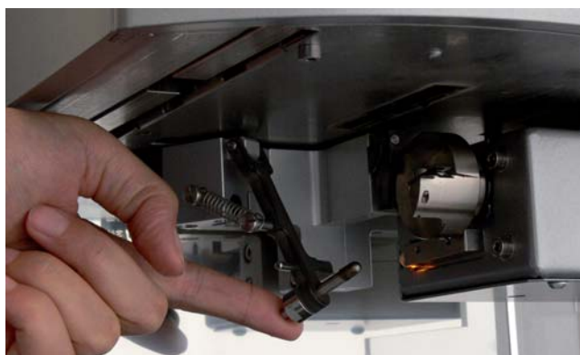
Fig. 4: The die plug prevents premature flow of the granulate
