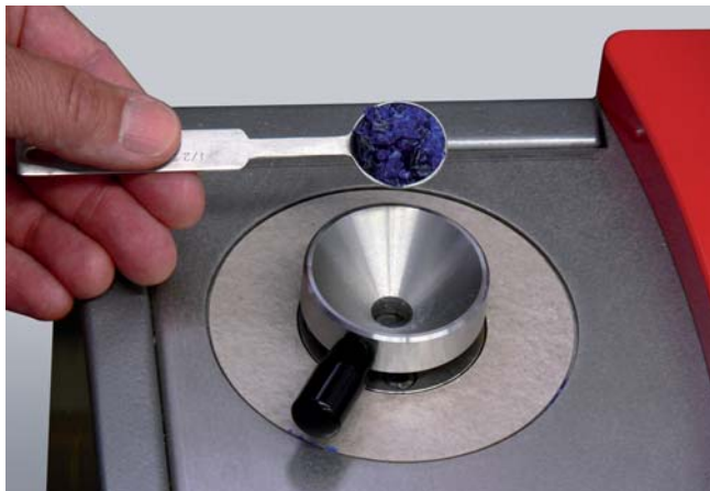
Fig. 2: Simple filling of granulate with the aid of the portioning measure and the specimen hopper
