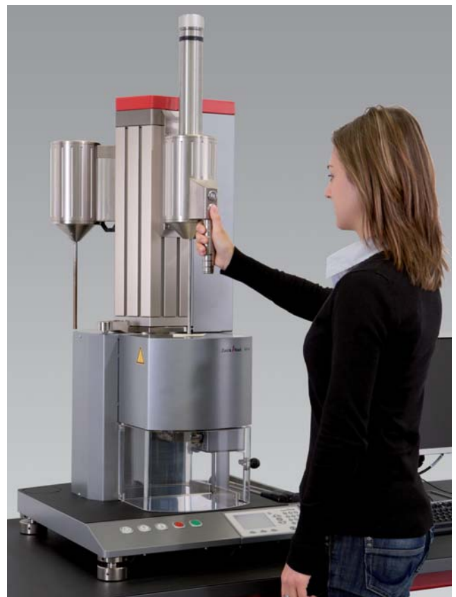
Fig. 2: Aflow: Cleaning and pre-compacting at the press of a button
