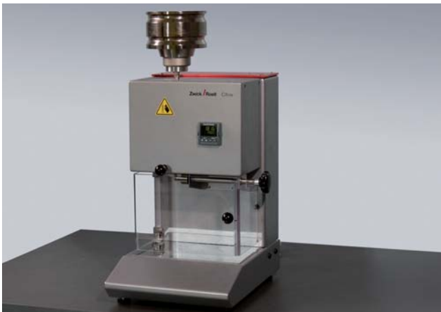
Fig. 1: The Cflow extrusion plastometer - precise MFR testing
