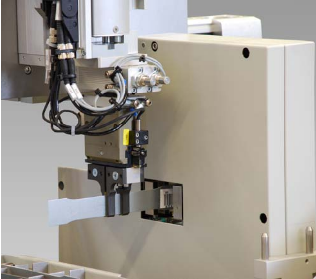
Specimen feeding to the cross-section measuring device
