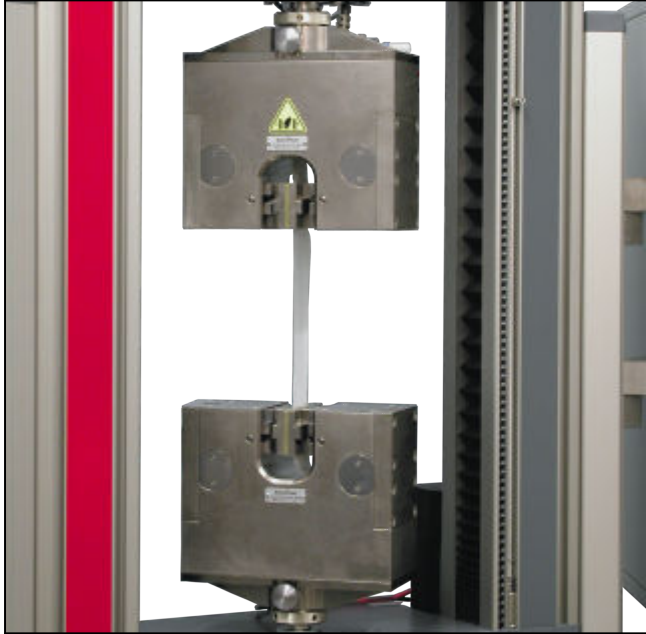
Pneumatic grips type 8497, F_{max} 20 kN, with high closing force
