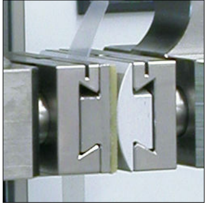
Jaws, convex aluminum against smooth vulkollan
