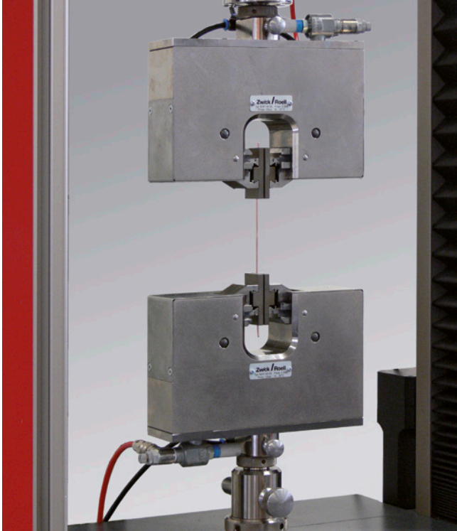
Pneumatic grips type 8297 with jaws height 50 mm
