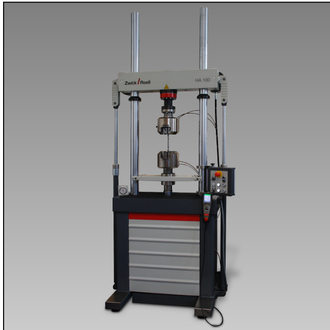
HA 100 on air springs with hydraulic wedge-grips
