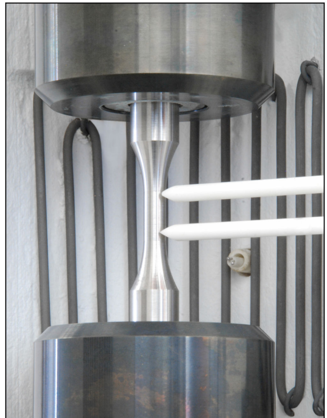
Specimen plus extensometer in high-temperature furnace
