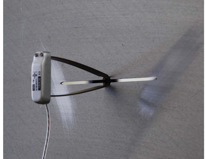
Extensometer on a middle-crack tension specimen
