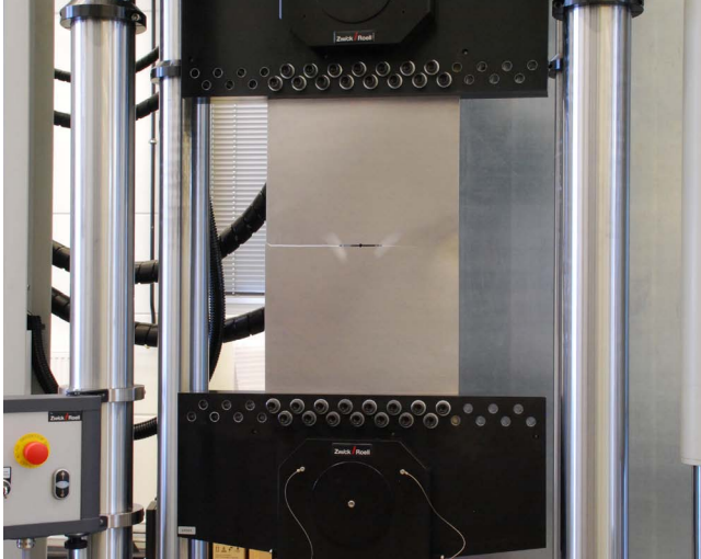
Middle-crack tension specimen installed
