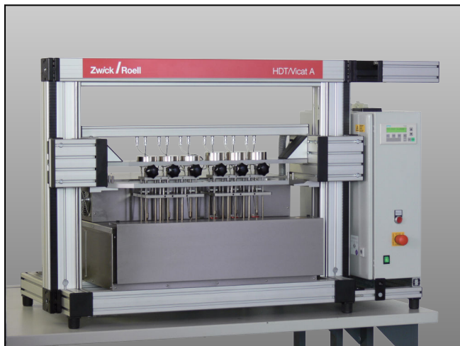
HDT/Vicat 6-300 Allround with motorized test weight application
