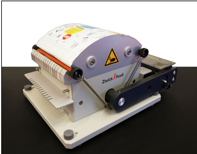
Strip-cutter for plastic film
