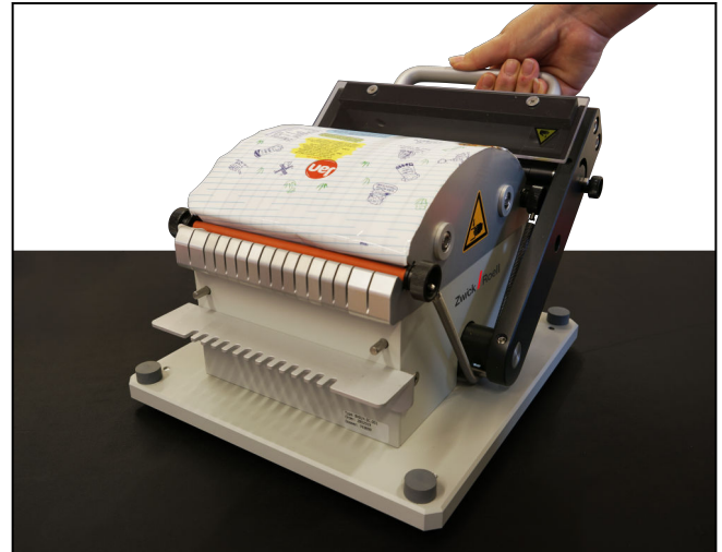
Strip-cutter for plastic film
