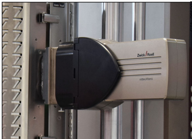
videoXtens 1-32 HP/TZ with optical tunnel on high-temperature furnace
