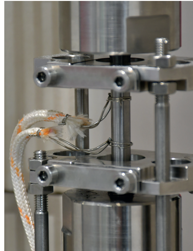
Creep test on metal specimen with contact-type extensometer
