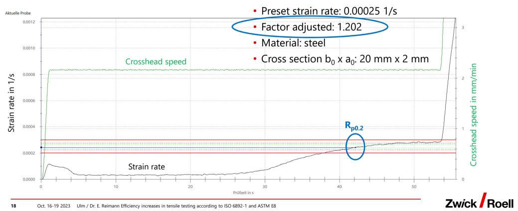
testXpert test program to ISO 6892-1: Method A1 (with yield strain)
