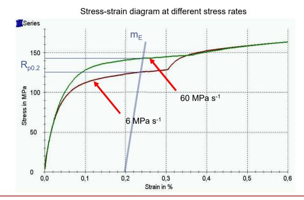
Reason: Metallic materials behavior is depending on testing rates, i.e. strain rates.
