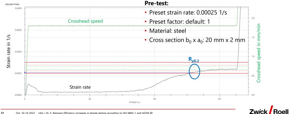
Test Method to DIN EN ISO 6892-1 Method A2 (valid test)
