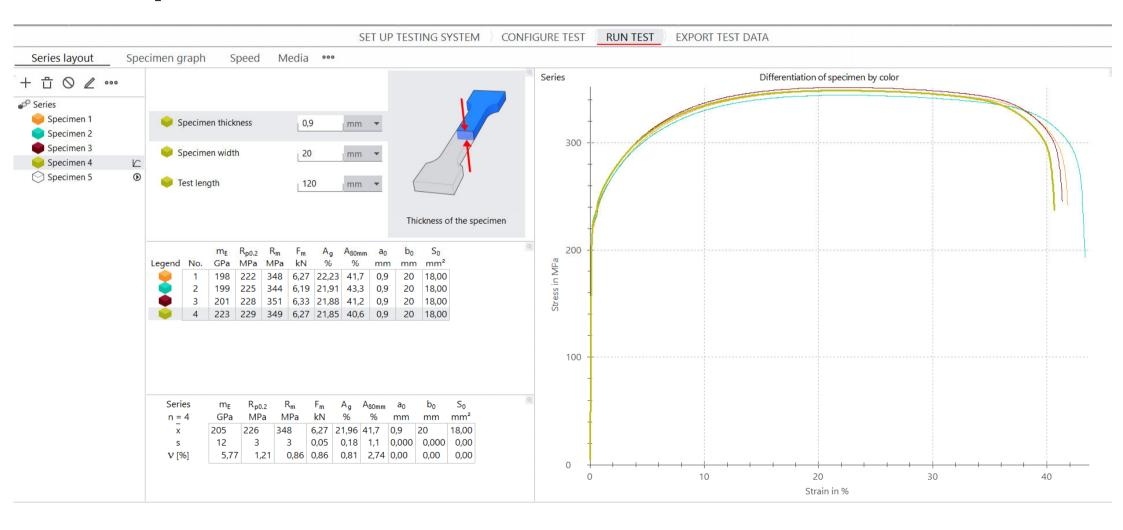
Typical test results to DIN EN ISO 6892-1 Method A1 – strain speed control
