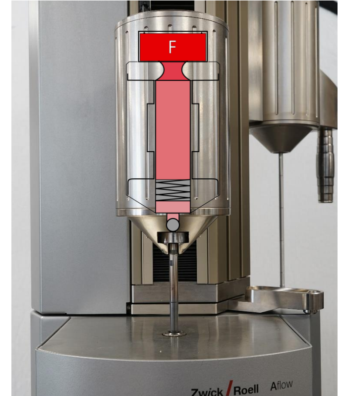
The force-controlled load apply system in an Aflow Melt Indexer is well protected against overload and temperature.
