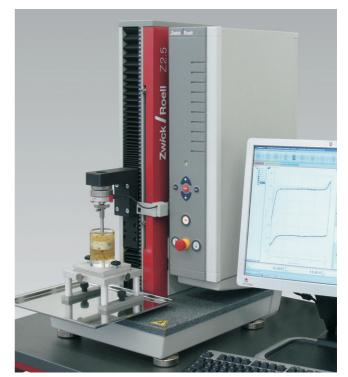
Fig. 2: Thanks to the simple interchanging of tools and fixtures the ProLine Z0.5 can also be used for viscosity tests
