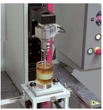
Fig. 1: Zwick Roell back extrusion rig
