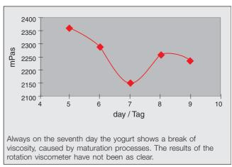
Fig. 3: Example for interpretation of viscosity tests on yogurt
