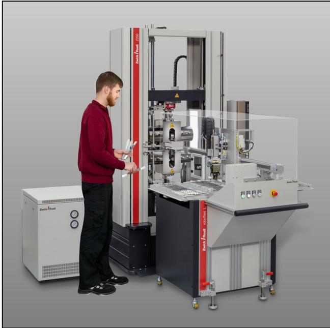
roboTest L robotic testing system for metals
