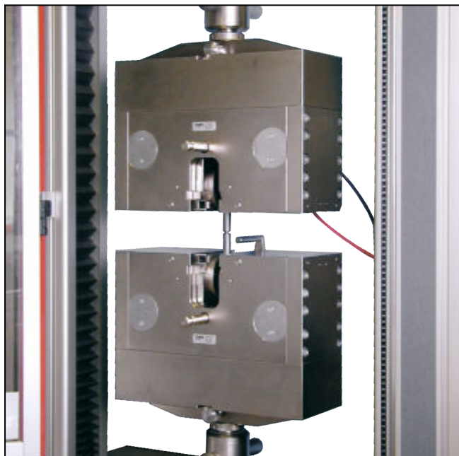
Pneumatic grips, type 8497, Fmax 50 kN
