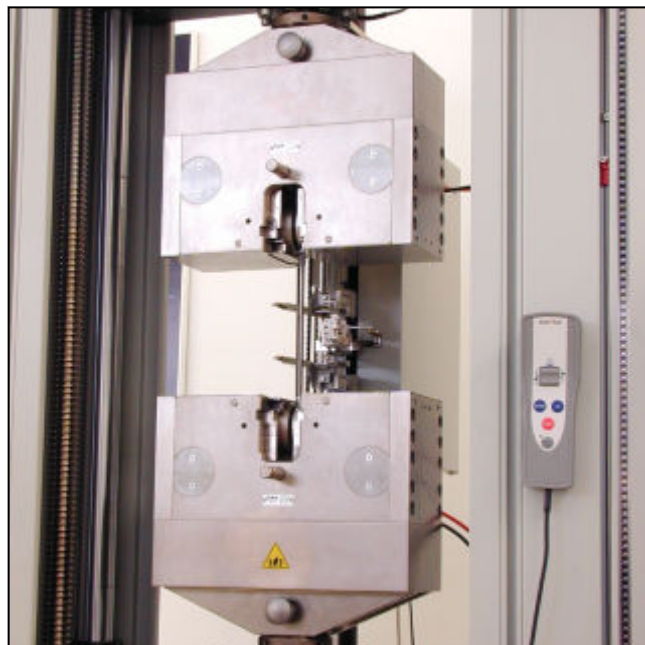
Pneumatic grips, type 8597, Fmax 100 kN
