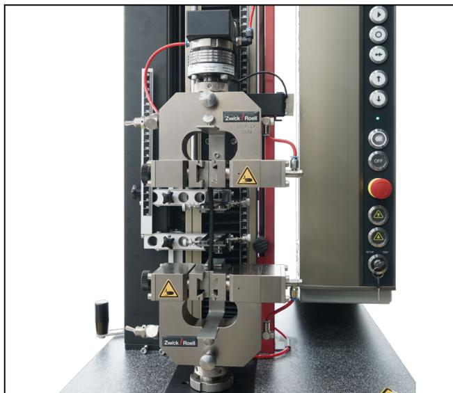
Pneumatic grips type 8195, Fmax 1 kN, with integrated control valve
