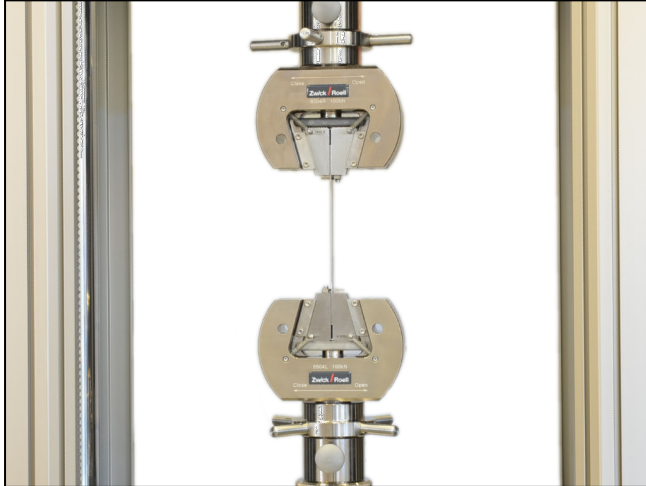
Wedge grips type 8504, Fmax 100 kN up to 250 °C
