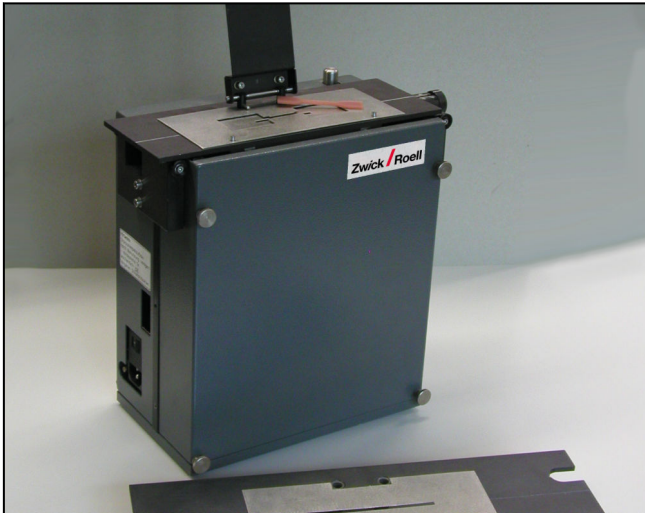
Automatic marking device, additional stencil for marking gauge lengths 50 to 100 mm
