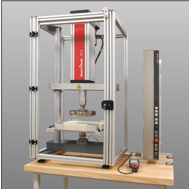
Dynamic fatigue test bench 5 kN
