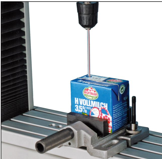
Vise (bottom) and clamping device for round specimens (top)
