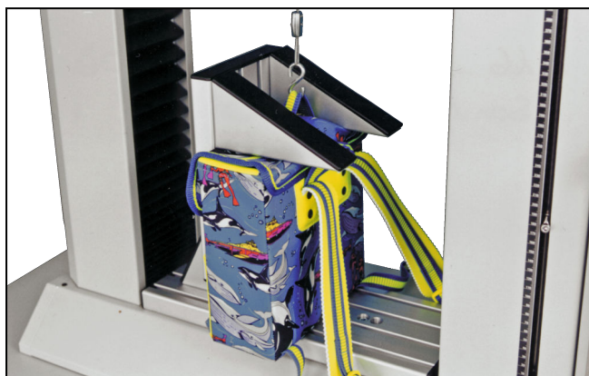
Angle bracket The T-slotted supplementary platform has been mounted on the T-slotted base platform using the angle-bracket. The angle bracket has also been used to clamp the satchel.
