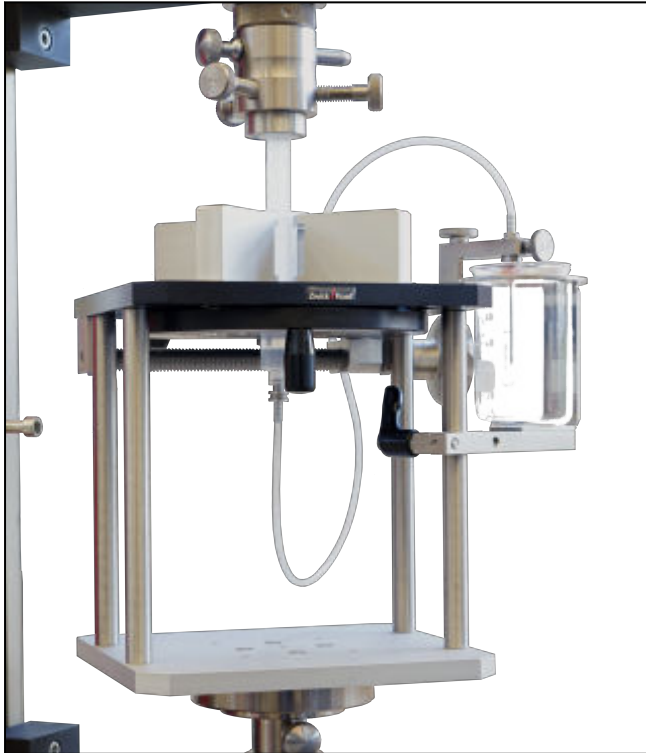
Test fixture for determination of plunger actuation force – Version 2
