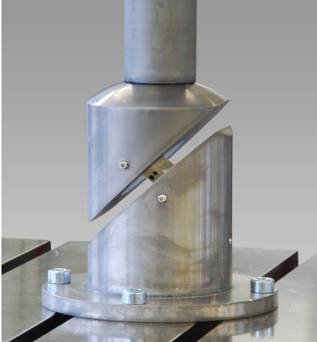
Shear test device with intervertebral disc prosthesis
