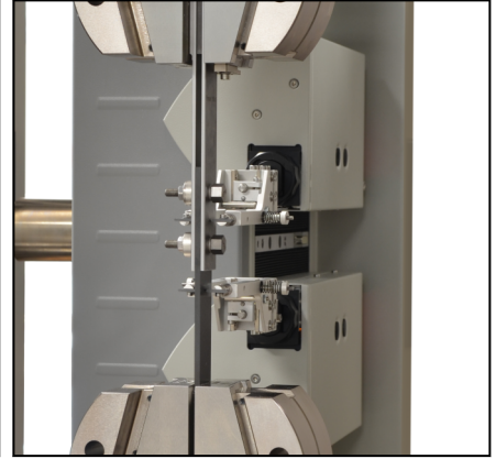
Bearing-strength test fixture as per ASTM D7248 Method A
