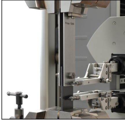
Bearing-strength test fixture as per ASTM D5961 Method A / ISO 12815
