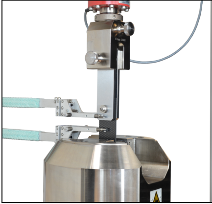
Bearing-strength test fixture as per AITM 1-0009 with specimen grips to hold the bearing-strength test fixture
