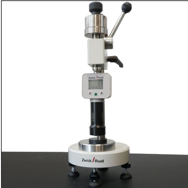
Digital ZwickRoell 3130 Hardness Tester to Shore
