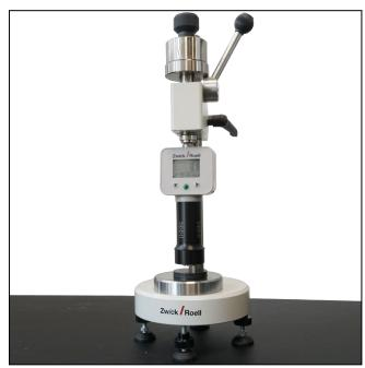
Digital ZwickRoell 3130 Hardness Tester to Shore
