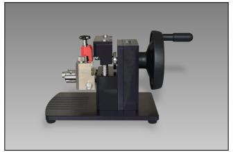
The removable specimen magazine makes it possible to notch four specimens simultaneously to ISO 179, ISO 180, and ASTM D256 and up to five specimens to ASTM D6110. In addition, more magazines can be prefilled; no extra tools or fixtures are required for this. The durable notch-cutter used has three cutting edges and can quickly be changed. Once the remaining width required by the standard is achieved, the blade is no longer fed and the specimens can be removed.
