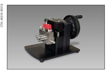
The notch cutting plane is designed solely for cutting notches in plastic specimens in compliance with the following standards:
