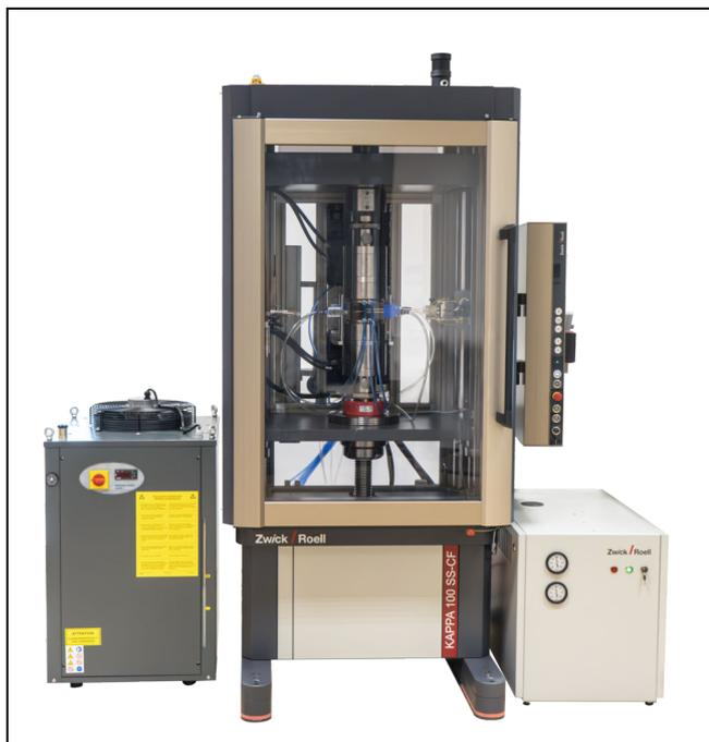
Thermomechanical fatigue testing system
