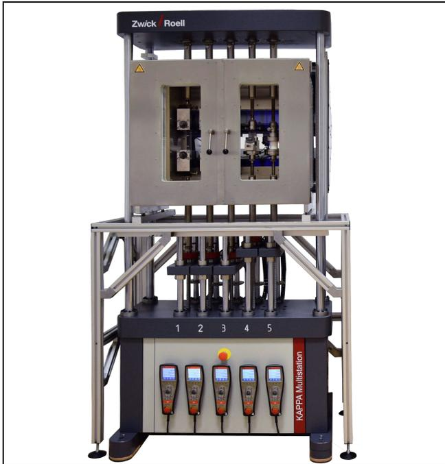
Kappa Multistation with five test axes
