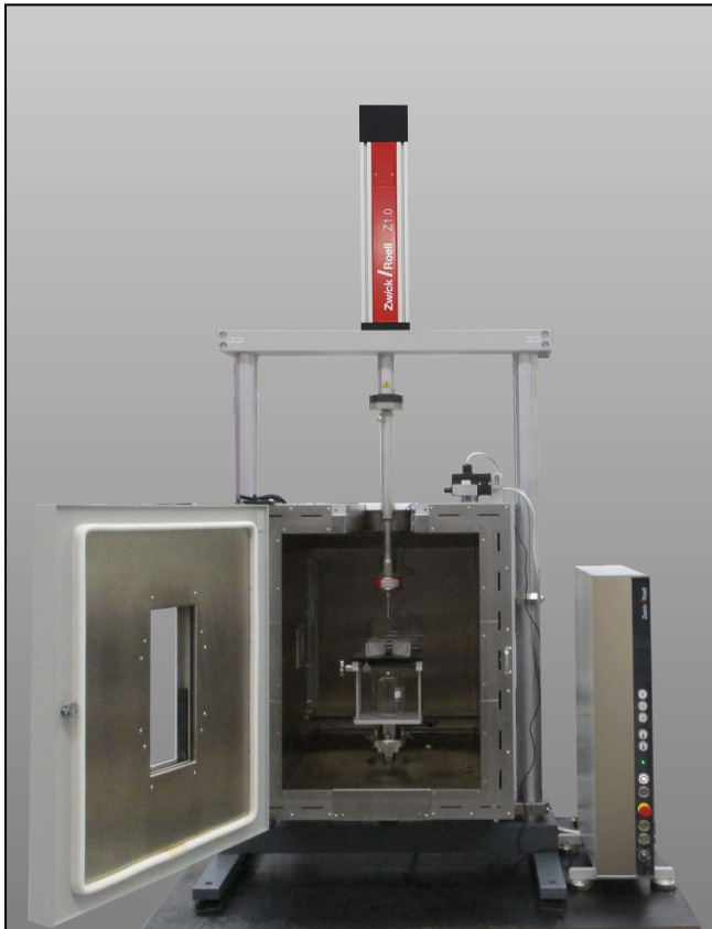
Electromechanical servo testing actuator 1 kN with temperature chamber
