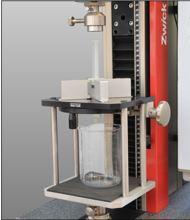
Test fixture for determining breakaway force and glide force
