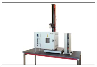
Temperature chamber for zwickiLine with optional large base (Item No. 059036) and optional leveling feet set (Item No. 083221)
